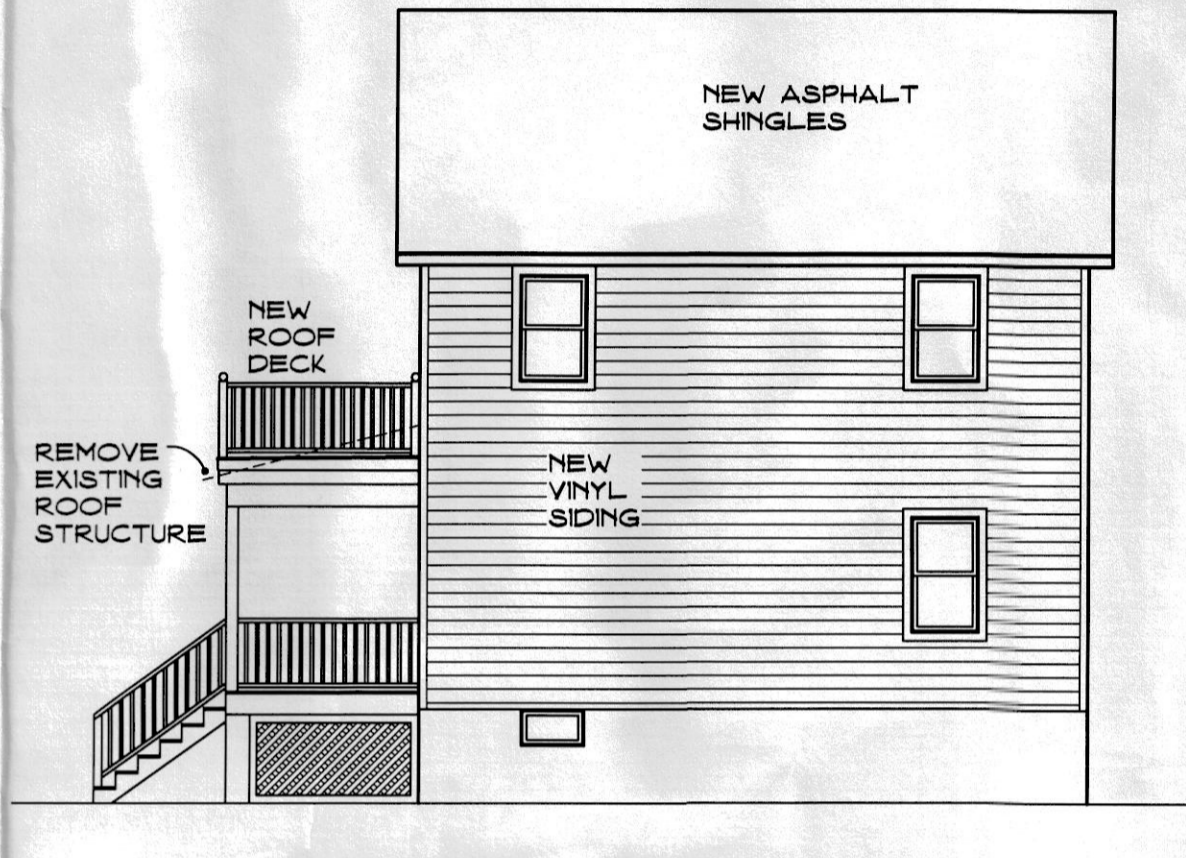
RIGHT ELEVATION SCALE 1/8" = 1'-0"
