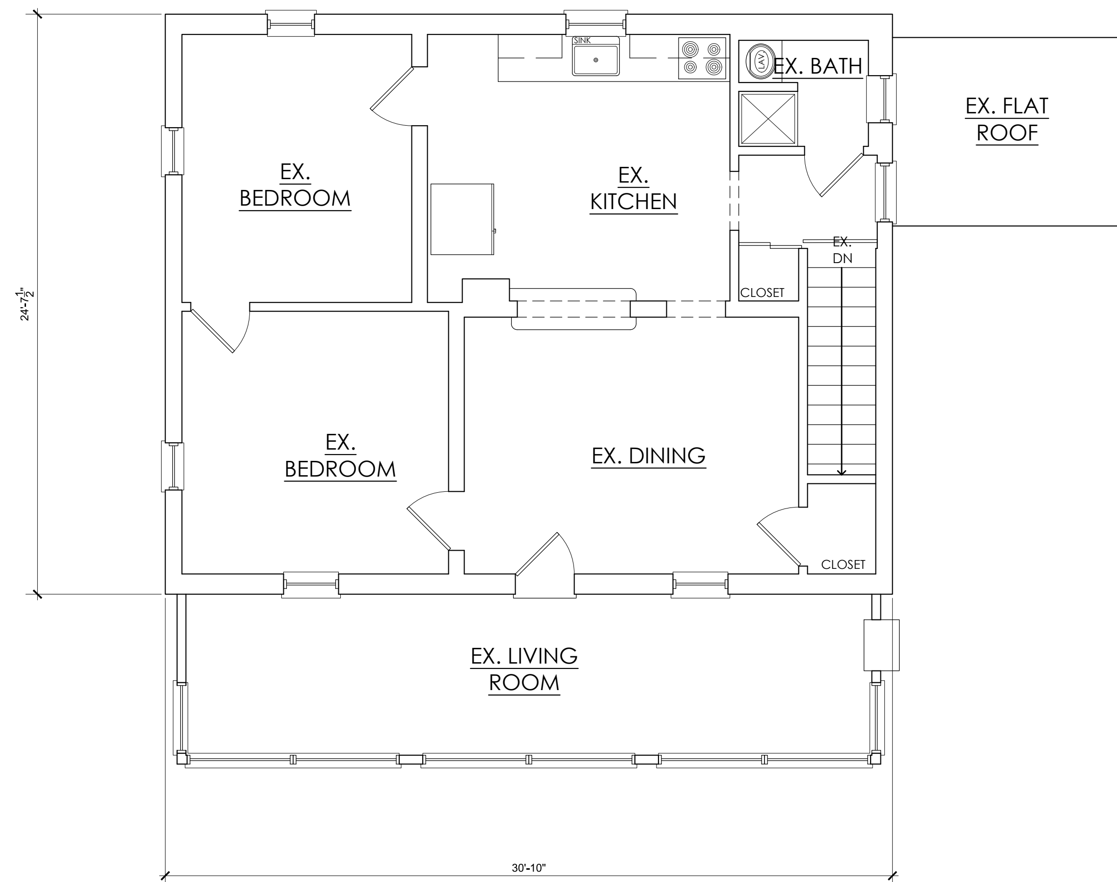
2 EXISTING SECOND FLOOR PLAN FLOOR AREA: 943 S.F. SCALE: 1/4" = 1'-0"
