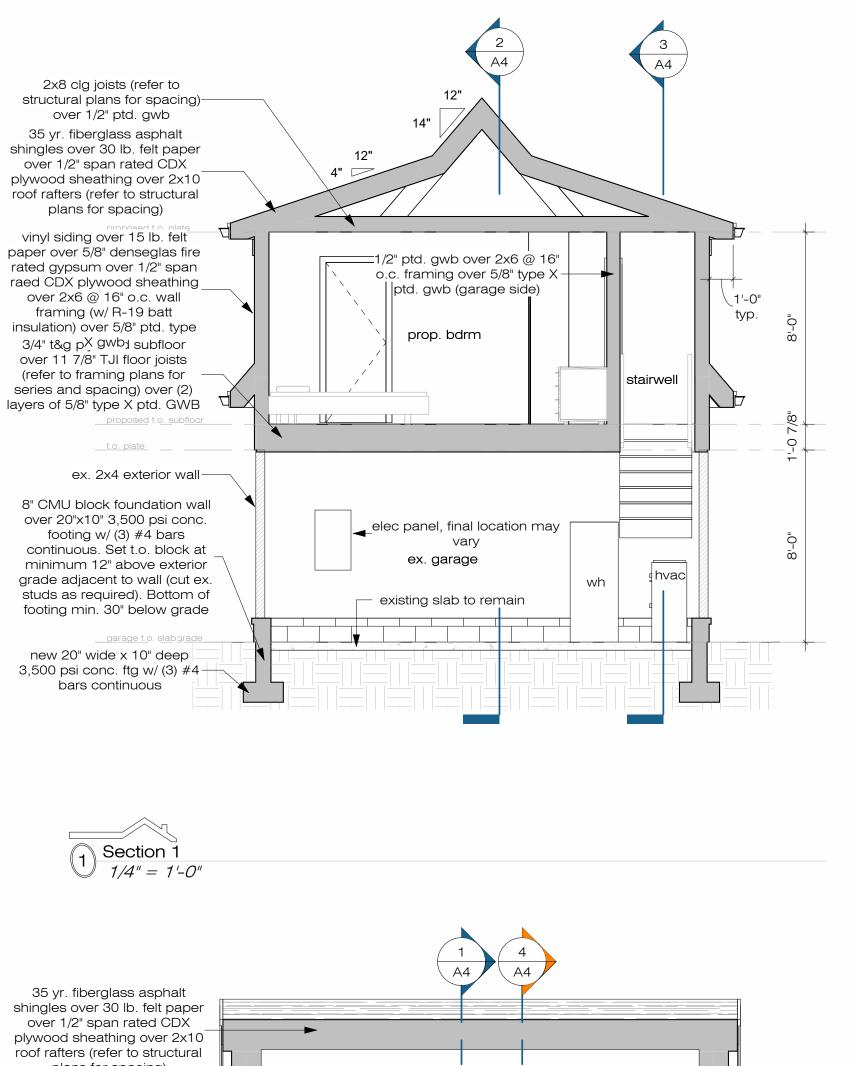
roof rafters (refer to structural plans for spacing) vinyl siding over 15 lb. felt paper over 5/8" denseglas fire rated gypsum over 1/2" span
