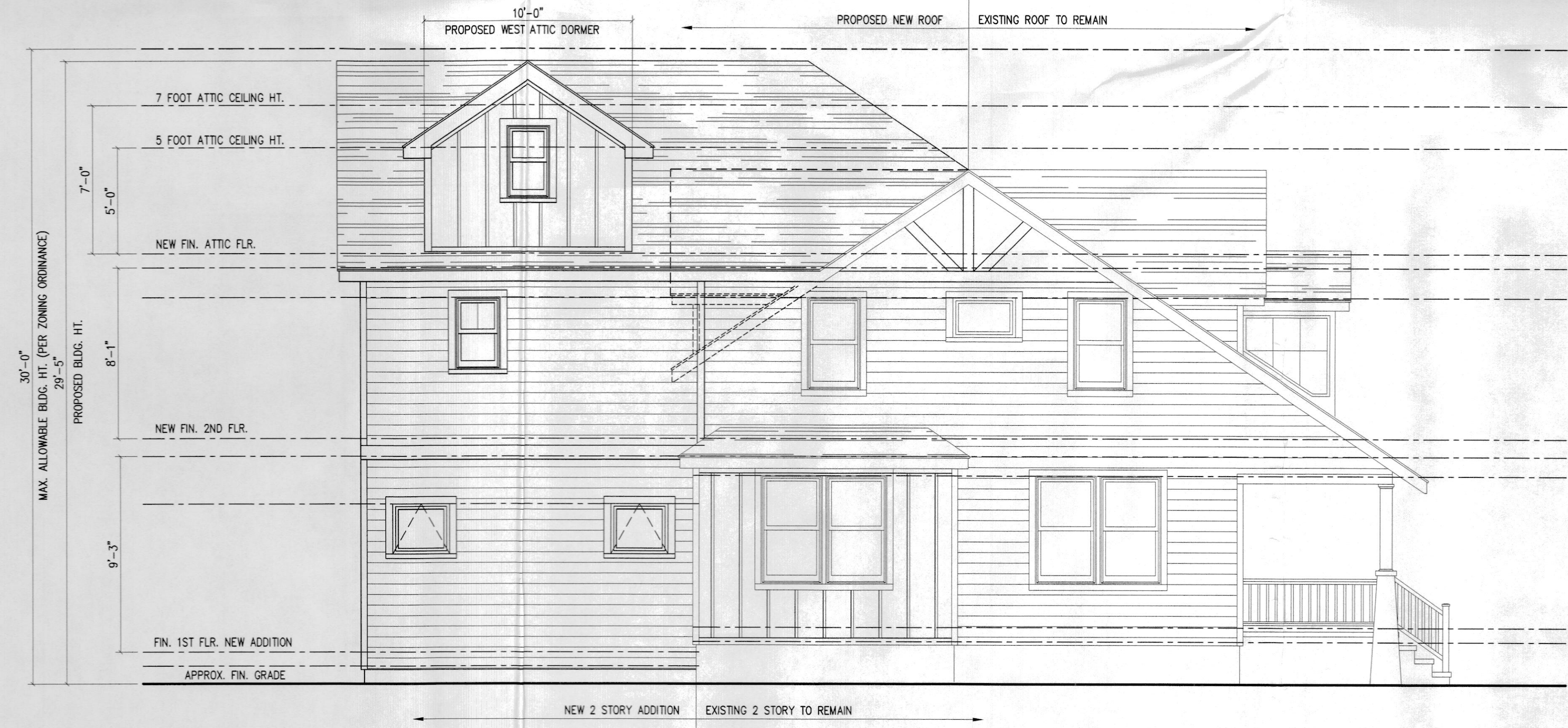
A Z-3 PROPOSED DRIVEWAY SIDE (EAST) ELEVATION SCALE: 1/4" = 1'-0"
