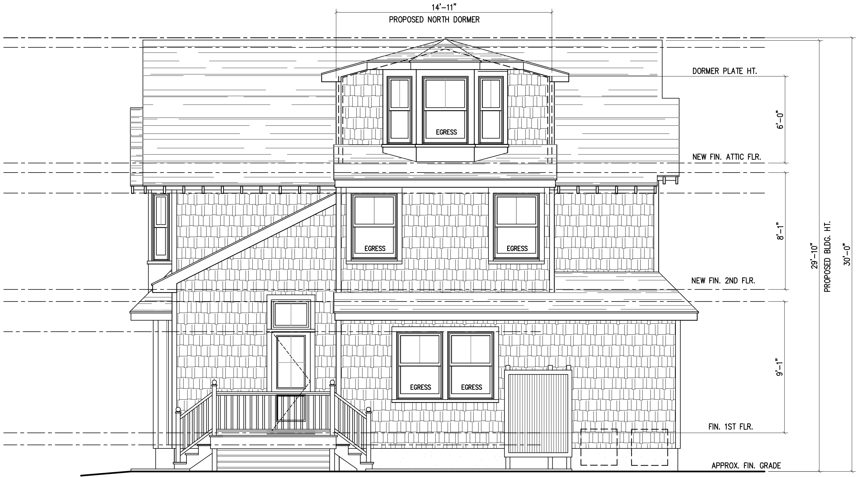
A Z-4 PROPOSED REAR (NORTH) ELEVATION SCALE: 1/4" = 1'-0"
